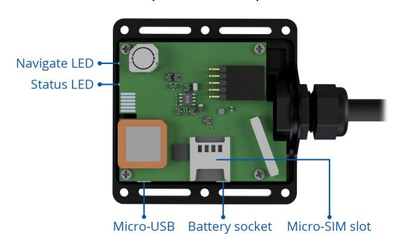
Figure 1 FMB204 device view
