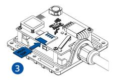
Figure 6 Micro-SIM card insert
