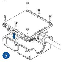
Figure 8 Attaching cover back
