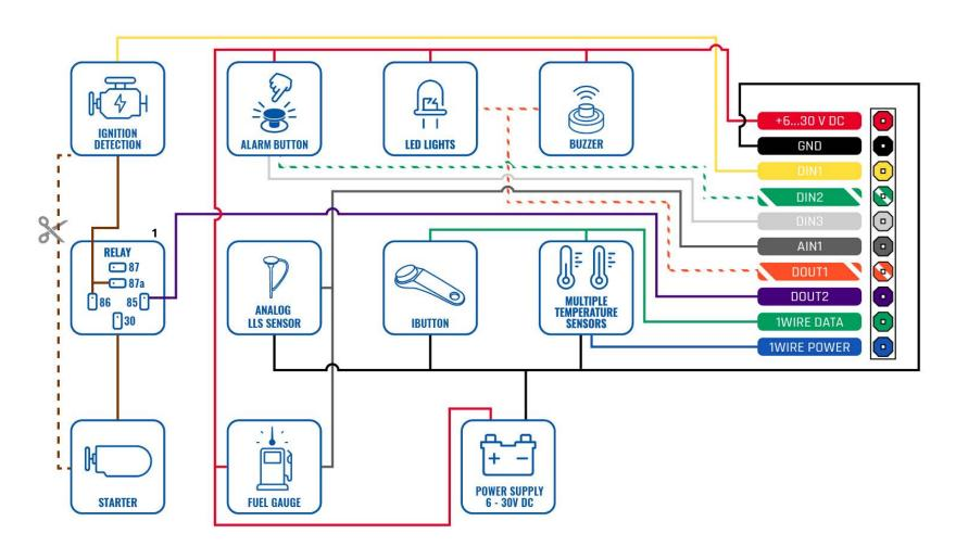
Figure 3 FMB204 Wiring scheme
